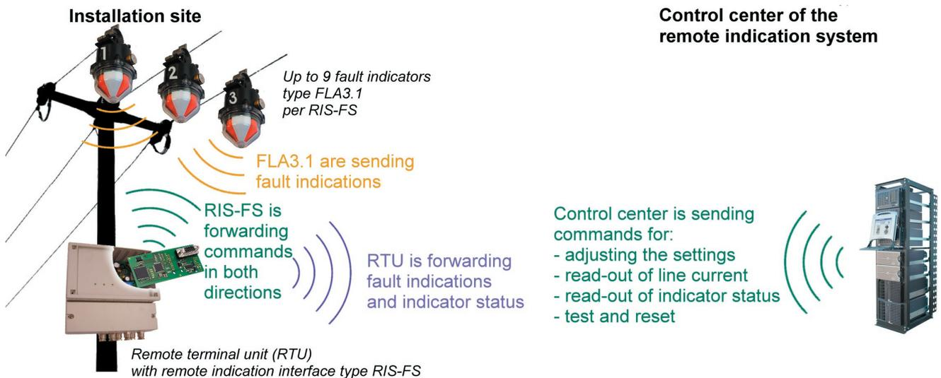
figure 3 - Installation scenario with fault indicators type FLA3.1
